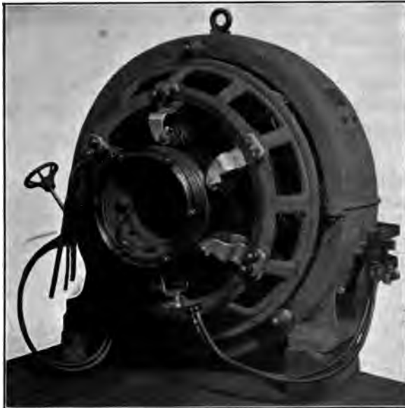
FIG. 27.—A 100 kilowatt, 250/125 volt, 260 r.p.m., three-wire generator manufactured by the Allis-Chalmers Co.
